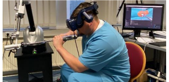
Fig. 8. A participant performing acetabula reaming using the Virtuoso 6D.
